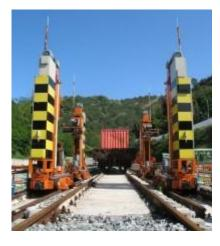
This solution allows the loading and unloading process of a whole train (to another train or to a truck) in one single automated operation without the need for any shunting activities. Photo: Metrocargo
